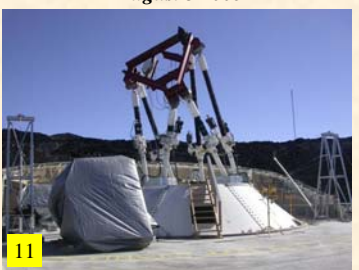
11 Dummy ring installation and testing for hexapod servo test February 24 2005
