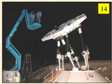
14 Photogrammetry measurements for the platform deformation verification September-October 2005
